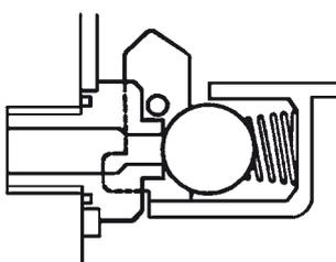
The Valve (Ball) lies inside a Valve Holder, which is directly connected through a lever with the float. By installing a spring inside the Valve Holder the movements of the float and the forces caused by it will not be directly transferred to the Valve. This will increase the service life of the sealing surfaces.
