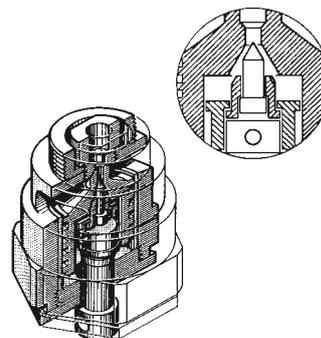
The SCCV®-System is part of a »Double Valve Unit«, which is operating on the basis of the pressure difference inside the unit. The trap is thus characterized by extended life of the valve assembly and a greater condensate discharge per body size when compared to conventional Inverted Bucket steam traps.
