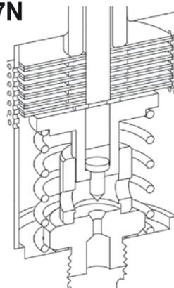
The Bimetal Unit including the Valve are guided inside the body. A spring reduces the force caused by the deflection of the bimetals which move the valve toward the seat. The guiding of the valve within the seat and the lift of the valve is designed in such a way that the Valve will close very smoothly in the center of the seat.
