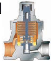
In case of very low condensate flow, the holes in the guide are closed completely by the valve holder and the valve will close precisely in the center of the seat. Normally, the trap is filled with hot condensate and the operation will rest in the state shown in figure 3. Condensate will be discharged continuously.
