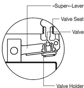
The Valve Holder is fixed to a specially developed »Super-Lever«. The Valve is »free floating« inside the Valve Holder. Thus the control space inside the Valve Holder decreases the force toward the seat caused by the movement of the bucket. The Valve will close softly and exactly in the center of the seat.
